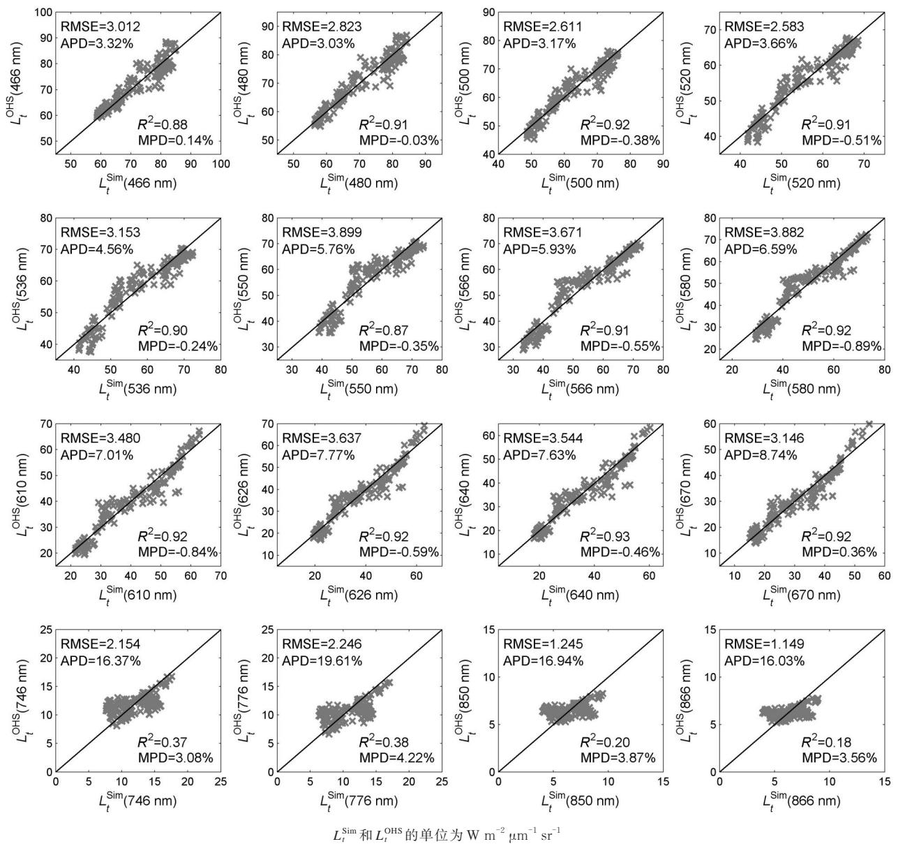
图9 新的定标结果  $L_t^{\text{OHS}}$  与模拟的  $L_t^{\text{Sim}}$  的散点图Fig.9 The simulated  $L_t^{\text{Sim}}$  values versus the new calibrated  $L_t^{\text{OHS}}$  values at different OHS channels
